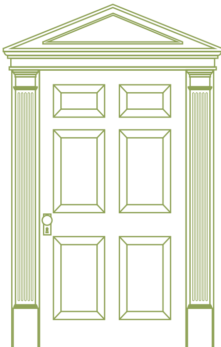
PEDIMENT + FLUTED PILASTERS
